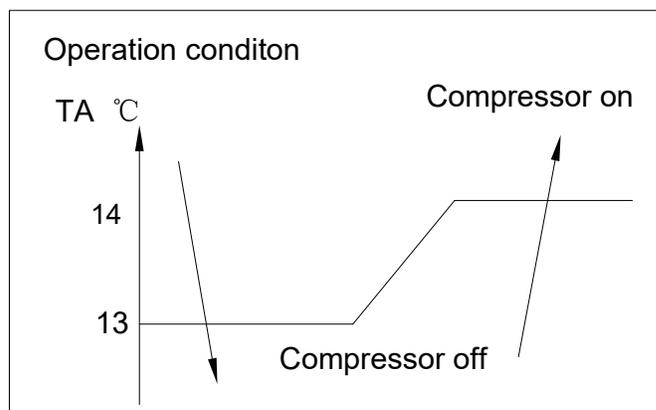
7.6.1.1 When  $TA < 13^{\circ}\text{C}$ , the compressor stops working. And the outdoor fan will stop delaying for 5 seconds until it operates for 3 minutes.
