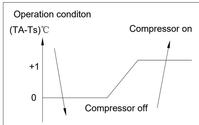
7.5.2.1 If  $TA > TS + 1^{\circ}\text{C}$ , the outdoor fan operates. After 15 seconds, the compressor operates.
