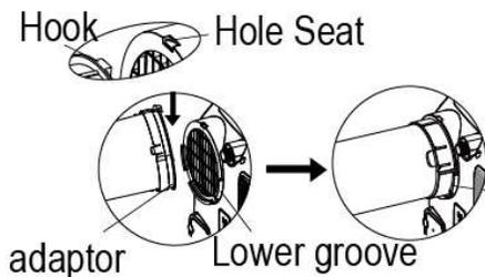
Make sure the adaptor is inserted into the lower groove of the air outlet.
