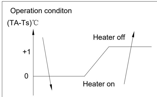
7.7.2.1. When  $TA < TS$ , the indoor fan operates firstly, and then the heater operates after 4 seconds.
