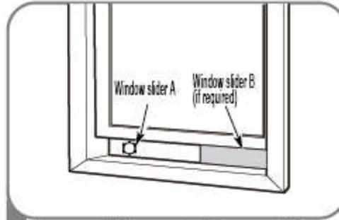
2 Insert the window slider assembly into the window opening.
