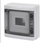
IP65 range of watertight anclosures from 8 to 72M with smoked transparent door and equipped with screw wiring multipolar terminal blocks, 80 A and IP20. The main technical features are: reversible front and back panel, removable frames and panels with windows and detechable doors with up to 180° opening and lock accessory. The terminal blocks allow to create simple and neat wiring reducing the set-up time of the enclosure.
